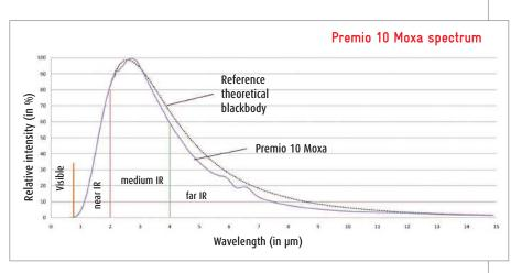
It behaves like an almost perfect black body, and, when in use, the emitter is stabilized at 850° C, and has a spectral peak to  $2,6 \ \mu m$ .
